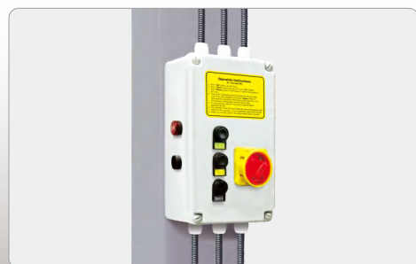
Electric control device With UP , LOCK and DOWN buttons With C.E. stop switch at 300mm from ground and alarm tone when lowering down from 300mm to ground make the lift more safety.
