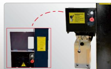
Optional Motor protective cover (with emergency stop switch) Kit No.:40810
