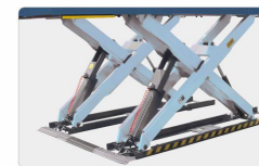
Two groups of total 4 hydraulic cylinders are intergrated to assure the equalization and safety of both platforms. (For X550/X550A/X730A)
