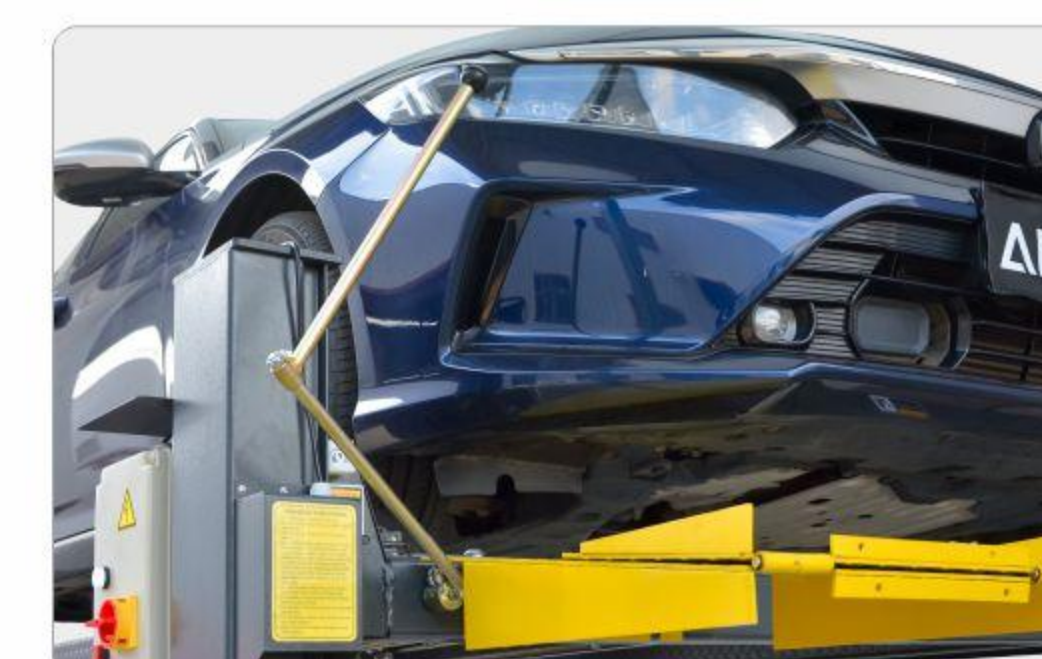
Patented concealed safety lock control with single-point manual release.
